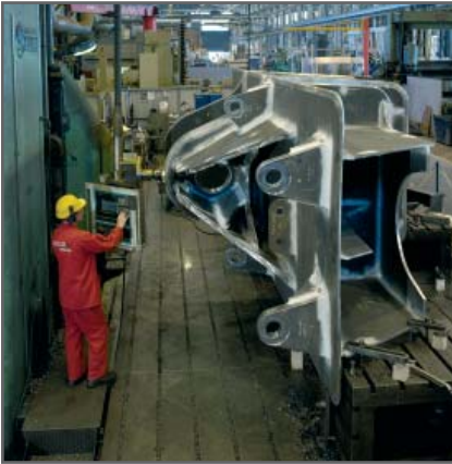
Machining of fairlead support for spar hull
