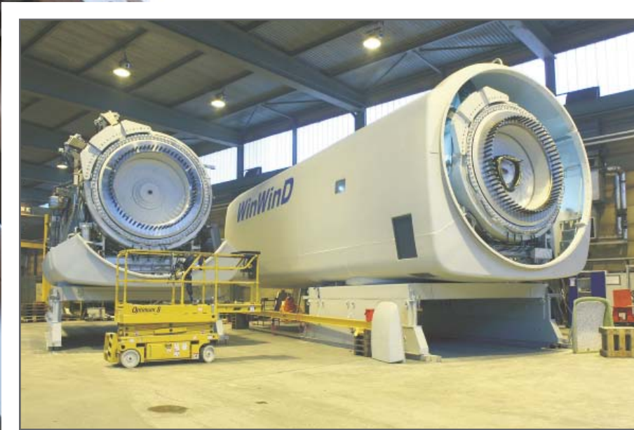
Nacells on assembly hall
