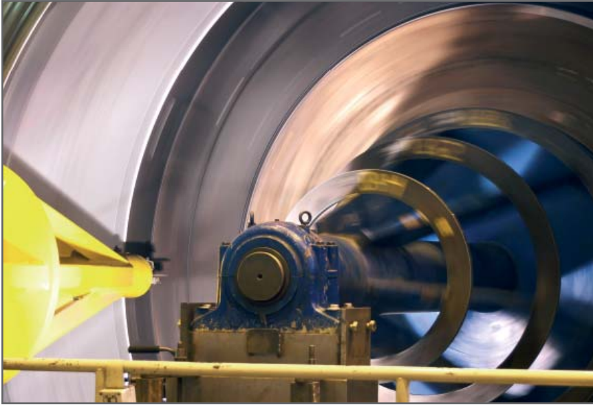
Special machine for machining e.g. stator and generator frames
